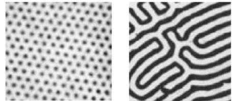
Figure 1: Laboratory type-II and intermediate type-I superconductor (Brandt & Essmann, 1987).
