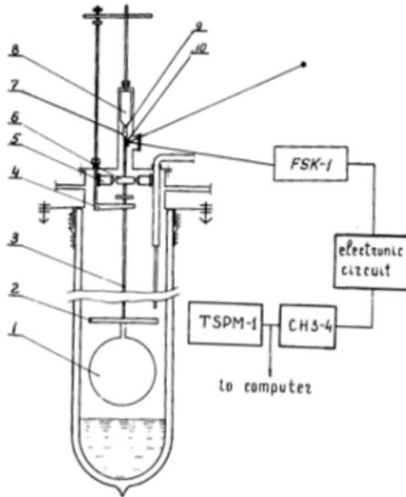
Figure 13: Schematic setup of the helium II spin-up experiments (Tsakadze & Tsakadze, 1980).
